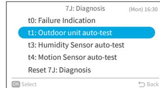
Step2. Select "Yes" and press "OK" to request outdoor unit auto-test. Then it returns to Step1.
