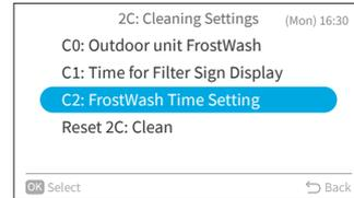
Step2. Press "^" or "v" to change the indoor unit auto FrostWash startup time, then press ">" to select "OK" and press "OK". Then it returns to Step1. Adjustment value of cumulative air conditioner time until execution of indoor unit auto FrostWash is as follow.
