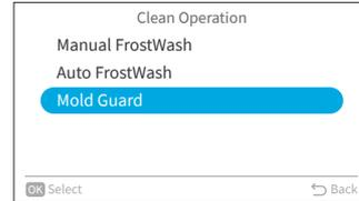
Step2. Press "v" to select "Enable" and press "OK" to enable the mold guard.
