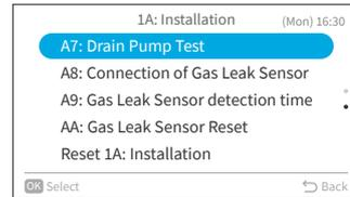
Step2. Select "Yes" and press "OK" to start drain pump test.
