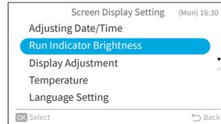
Step2. Press "^" or "v" to change the brightness value. Select "OK" and press "OK", the screen returns to the "Screen Display Setting" screen.
