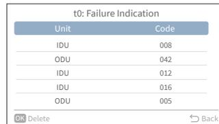
Step3. Press "OK" and a reminder shows up. Select "Yes" and press "OK" to delete all failure logs.
