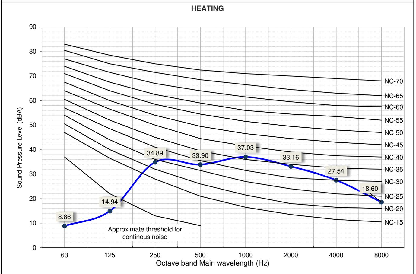
The Sound Pressure Level is based on the following conditions:
