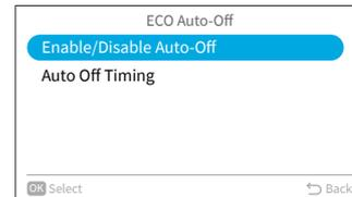
Step3. Press "^" or "v" to select "Disable"/"Enable" and press "OK" to enable/disable Auto-Off.
