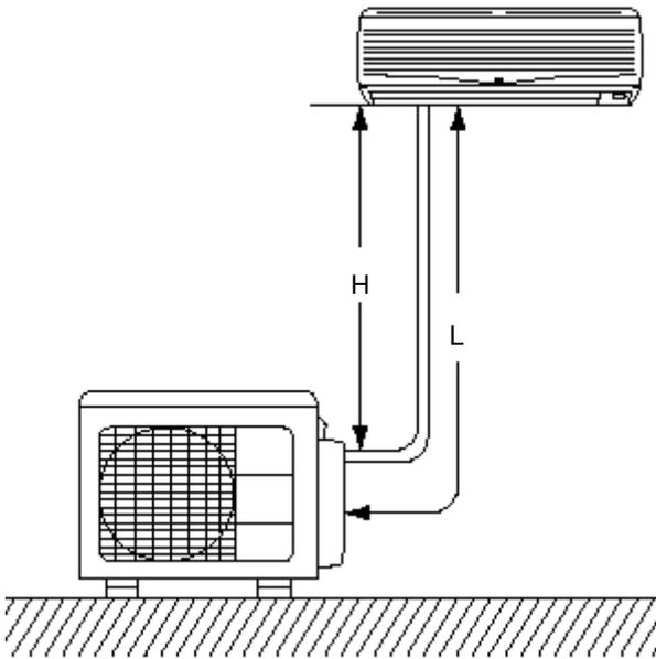
H: Vertical Distance Between Indoor Unit and Outdoor Units in Meters
