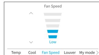
Step2. By pressing "^" or "v", the fan speed changes as follows.
