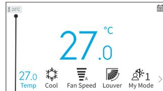
The icon indicates that the thermistor temperature is set to be displayed.
