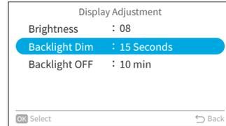
Step3. Press "^" or "v" to select the dim time intervals and press "OK". The item changes as follows:
